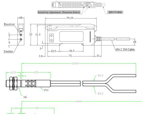
Fiber Optic Cable Diffused Beam Model: FOS100D, Sn: 100mm
