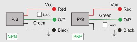
Sensor can be used to drive 12 VDC/ 24 VDC Relay, can be coupled to PLC, Digital Counter, RPM indicator etc.
