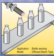
This device consist of a transmitter and a receiver together. This look alike Inductive Proximity Sensor and hence also known as IR Proximity Sensor. The emitter emits Infra red rays which are reflected on the receiver through the object to be registered. In the use of these sensors, it is important to bear in mind the colour of the object. Light colour corresponds to the maximum distance and vice versa. In case of shiny object; the effect of surface of object is more important than the colour.
