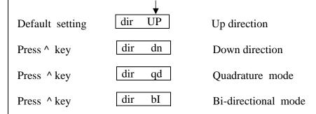
4)Press ACK to program **Reset selection** .This feature can be used only in quadrature mode and bi-directional mode.
